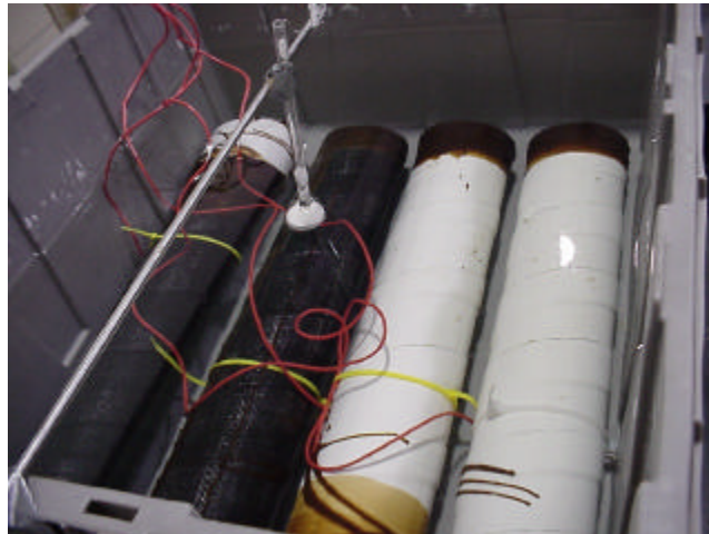
Figure 3. The four 18-inch long, 3 inch diameter pipes coated in either RD-6 or 610 coatings and submerged in 3% NaCl solution for Task 2.
